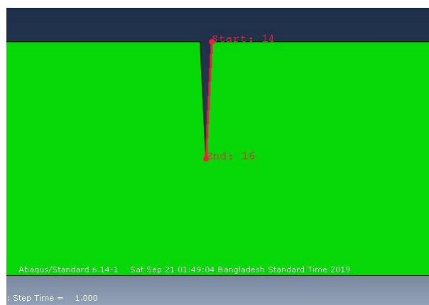
Figure 5. Path along the crack
